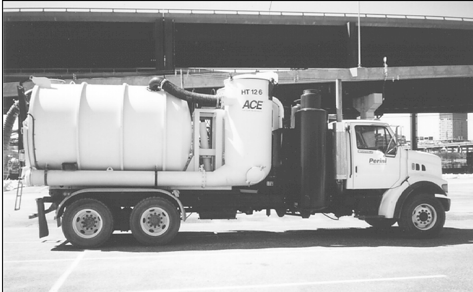
FIG. 1. Vacuum Excavator Truck
