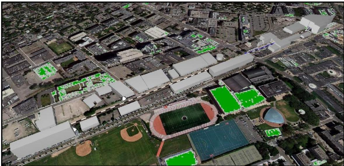
**Figure 3. Cadna-A Noise Model Configuration**
