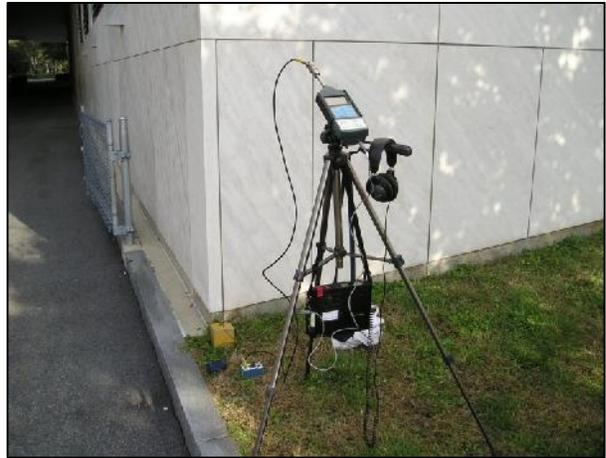
**Photo 4. Vibration Monitoring Equipment**
